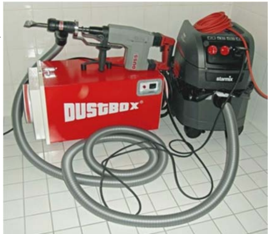
Figure 8: Sucked off hand-held tools (here a demolition hammer), construction dust collector and air cleaner. To meet requirements, the minimum equipment with low-dust techniques does not even cost 3,000 euro for each enterprise
